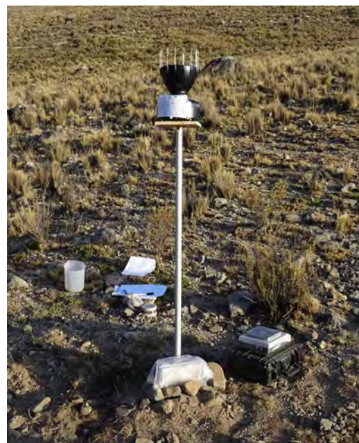
» Figure 2.4: Assessing soil hydraulic conductivity in the Lurín catchment using a hood infiltrometer (left). Rain gauge RSN05 in San Damián district at 4455 m asl (right). Pictures: J. Bondy.
