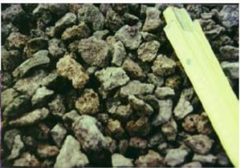
Topview of a trickling filter filled with lava rocks (Sindelfingen, Germany)
